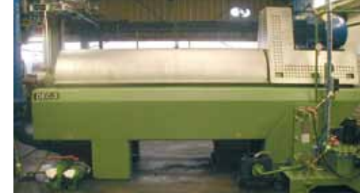
The 3-phase decanter CB 635 separates oil, solids and water in one work cycle.
