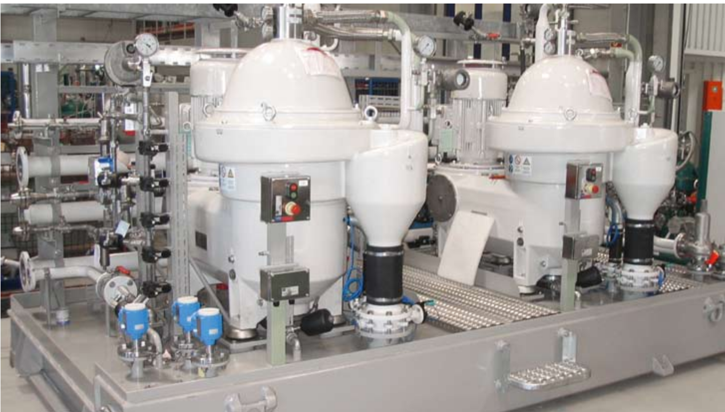
Double module with WSD 60 separators for oily water
