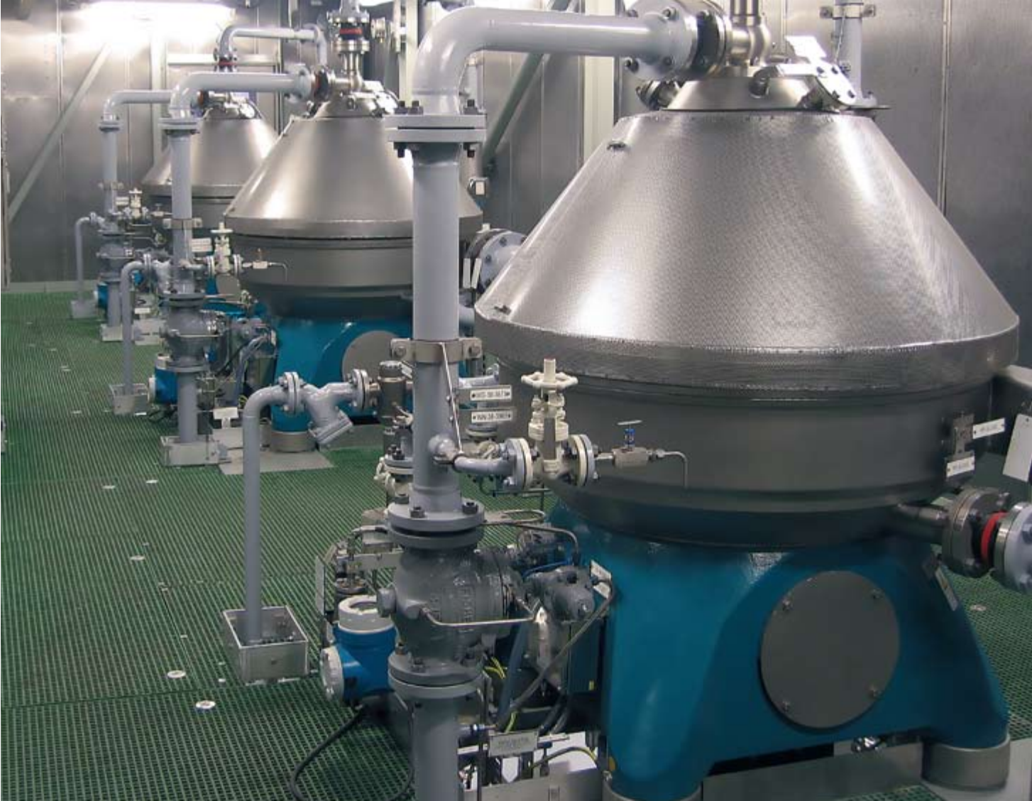
Triple module with WSD 200 separators for mono ethylene glycol clarification
